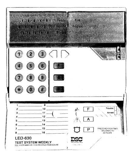
**ZONE** light(s) when ON in the normal operating mode indicates an open zone. eg. open door, window, etc. Refer to zone chart on keypad door for zone information.
